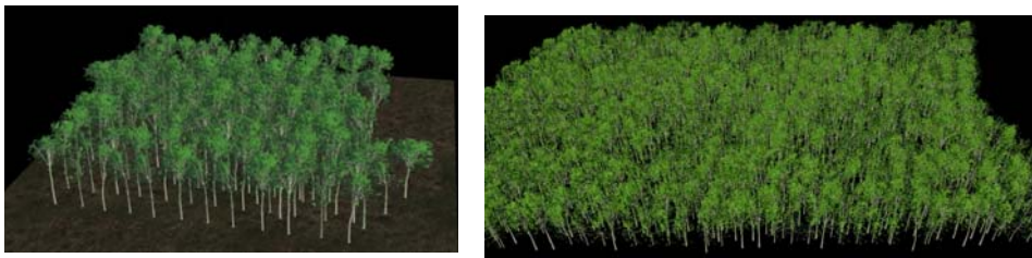
Figure 3. VRML forests generated automatically from individual tree scenes. 120 single trees rendered as billboards (left) and 3000 trees rendered using low cost geometrical models (right)
